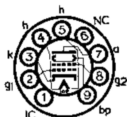
The BRIMAR type 6061 is a B9A (Noval) based output beam tetrode, the characteristics and ratings of which are identical to those of the 6V6G/GT. It is suitable for R.F. applications up to frequencies of the order of 150 Mc/s.
